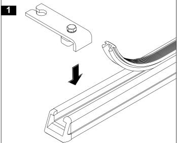
Locate the channel nut into the crossbar recess, turn the attachment bolt so that the channel nut rotates and locates across the crossbar. Adjust the position of the bracket and tighten the attachment bolt. Check that the channel nut is fully located across the crossbar after tightening. Trim rubber buffer strip to suit.
