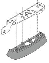
Locking points push through and fix onto Bracket.
