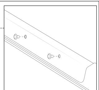
Install the Leg Bracket onto the Rubber Skirt.
