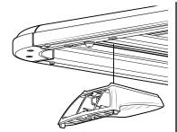
Attach leg assemblies to the Pioneer underside bars. Tighten leg hardware to a firm <u>sliding</u> fit.
