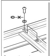
Remove the spring washer from the button head and channel nut assembly of the Pioneer underside bar. Re-install button head with flat washers only.
