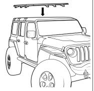
Place Pioneer assembly onto RJLB1 castings. Slide legs into position and attach to castings. Centre Pioneer between legs and tighten all hardware to final torque.
