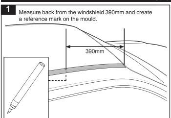
Lift the ditch mould out from the rear, stopping at the reference mark made previous, 390mm back from the windshield.
